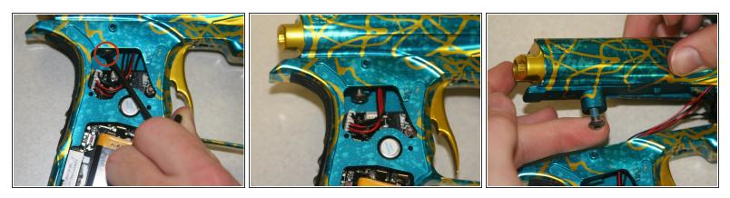
Use 1/8" allen wrench to loosen the screw inside the grip on the right side.
