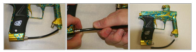
• While pulling in the metal ring on the fitting, pull the macroline out.
