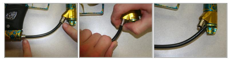
• Remove the macroline from the fitting by pulling the metal ring around the end of the fitting away while pulling out the macroline.
