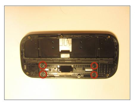
Use a screwdriver and corresponding bit to remove the four 1mm screws. Set the screws aside.
