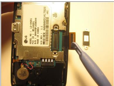
Use the plastic opener to disconnect the ribbon cable.
