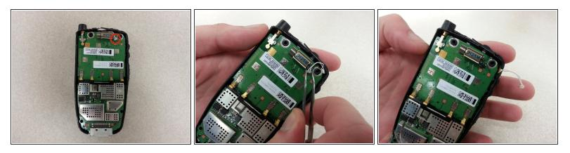
Using a pair of tweezers, firmly grasp the connector at the top of the phone and pull the connector straight away from the phone.
