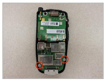
Using a Torx T8 screwdriver, remove the two circled screws by unscrewing counterclockwise.
