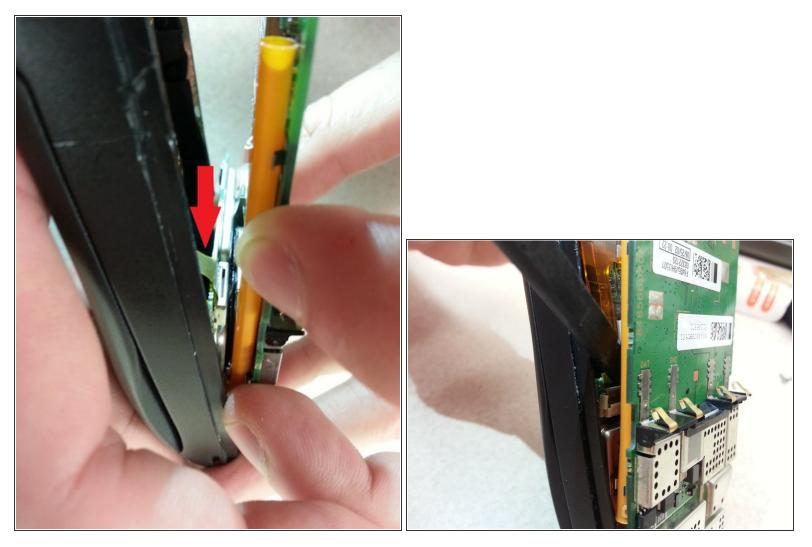
• Unclip the ribbon cable, located underneath the motherboard, by using the spudger to push up on the dark brown part of the connector located on the circuit board.
