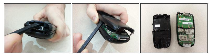
• Starting from the bottom and working towards the top, use a spudger to pry the back cover off the phone.
