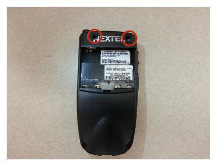
Using a Torx T8 screwdriver, remove the two screws exposed after removing the sticker by unscrewing counterclockwise.
