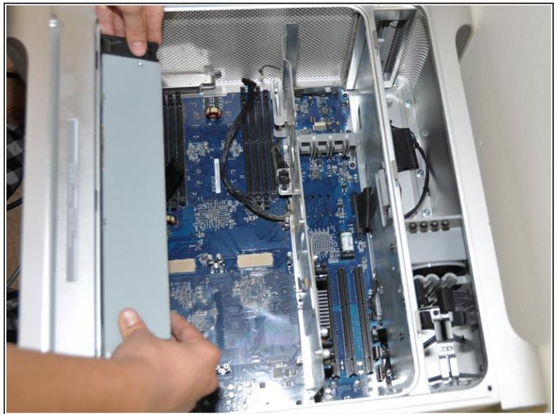
**i** Carefully pull the power supply out of the case.
