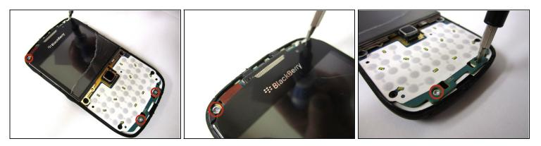
Locate and remove the four 5mm screws on the top and bottom of the phone with a T6 Torx screwdriver
