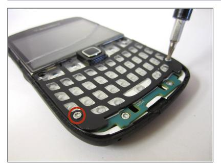
Locate and remove the two 5mm screws on top of keyboard base using the T6 Torx screwdriver
