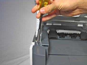
Locate and remove the two 10mm side screws. There is one on each side.
