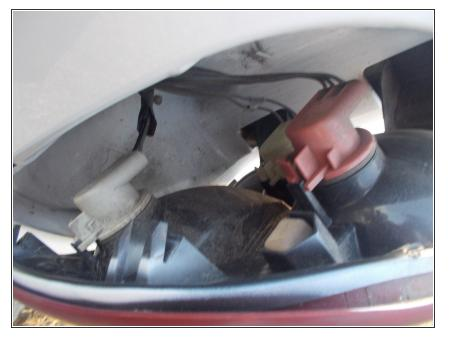
Once the screws have been removed, simply pull off the taillight. The red plug is the taillight. Twist it a quarter turn counter clockwise, and pop it out.
