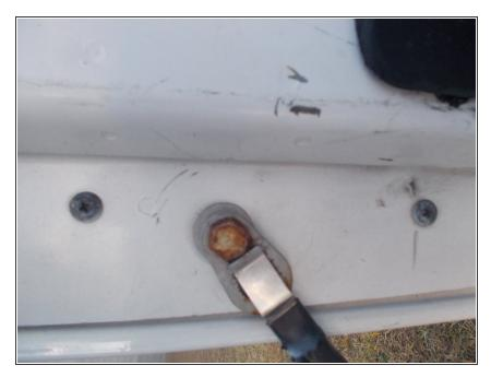
• Unscrew the two phillips head screws located above and below the tailgate support.
