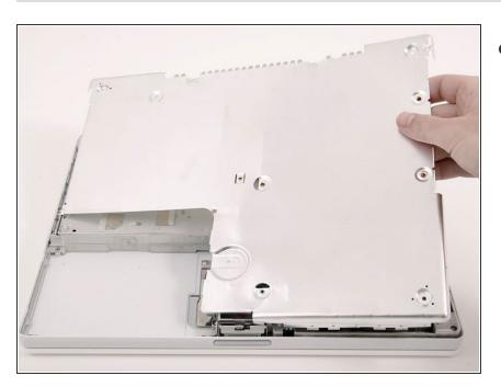
Lift the bottom shield off.
