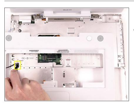
Carefully disconnect the multicolored speaker cable from the logic board. As before, make sure you're pulling only on the connector and not on the socket.
