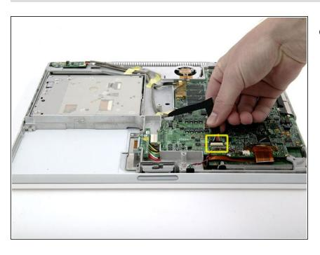
Disconnect the DC-In cable from the logic board.
