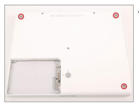
Remove the three newly-revealed Phillips screws.
