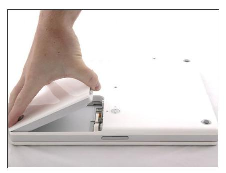
Lift the battery out of the computer.
