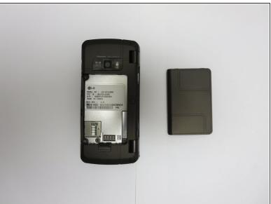
Lift the edge of the battery to remove it.
