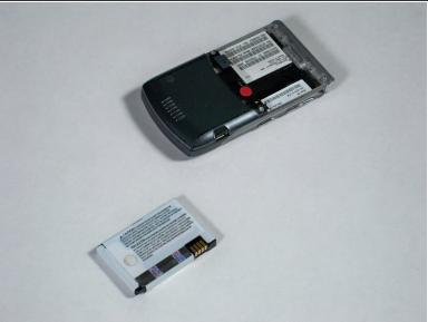
Remove the battery by pushing in the top of the battery and lifting it away from the phone.
