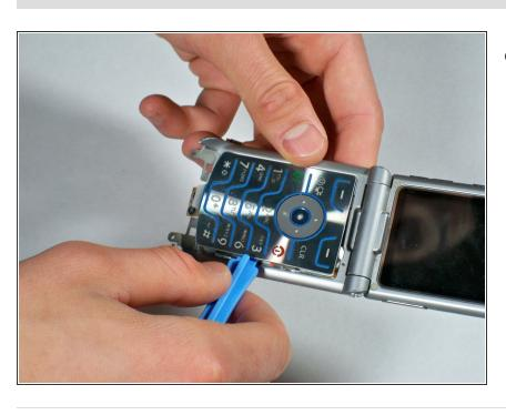
Gently lift up on the keypad with the plastic opening tool while being careful not to bend the thin metal portion lining the keypad.
