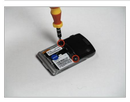
Remove the two T6 screws on the back of the phone.
