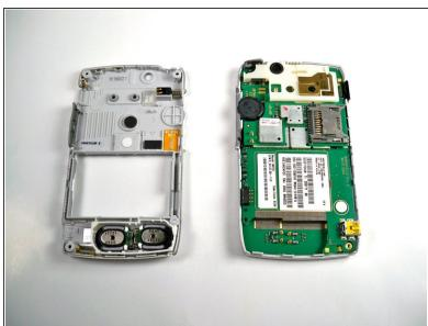
Gently lift and remove the back casing.
