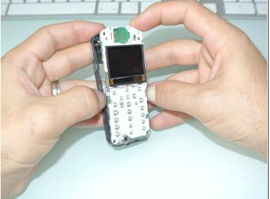
Use a metal spudger to pell off the four metal clips and separate the motherboard and keyboard from the main plastic part.
