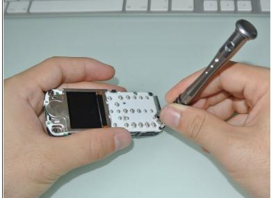
Remove the four T6 Torx Screws
