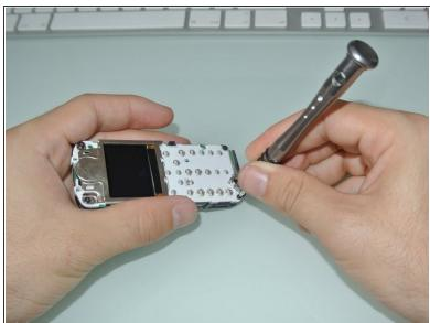
Remove the 4 T6 Torx screws
