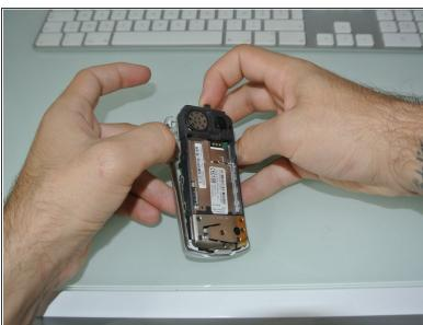
You will see one plastic clip on each side of the device. Use your thumbs to push them apart and being able to separate the front case from the device other components.
