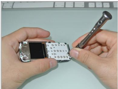
Remove the four T6 Torx Screws
