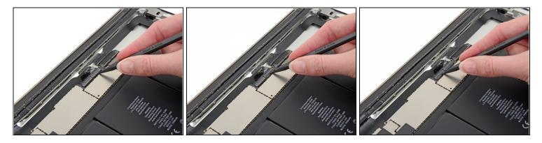
• Flip up the retaining flap on both of the digitizer ribbon cable ZIF connectors.
