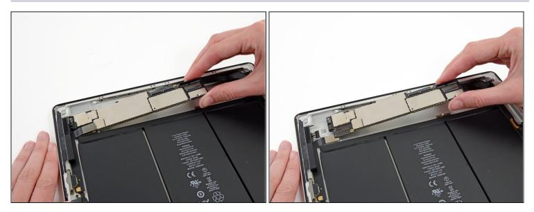
• Holding the logic board by the side opposite the Lightning connector, carefully pull the logic board away from the iPad.
