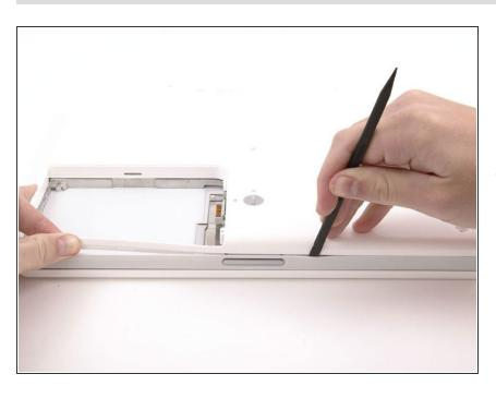
• Run a spudger along the seam between the lower case and upper case on the front of the computer to free the tabs locking the lower case. Pull up on the lower case and continue to use the spudger as necessary until you hear three distinct clicks.
