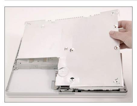
Lift the bottom shield off.
