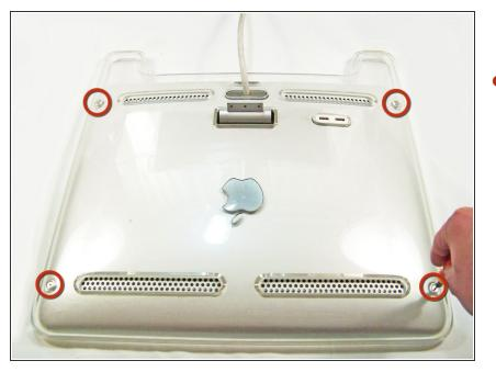
Remove the size 2.5 hex screws from each corner that connects the panels to the display and remove them.
