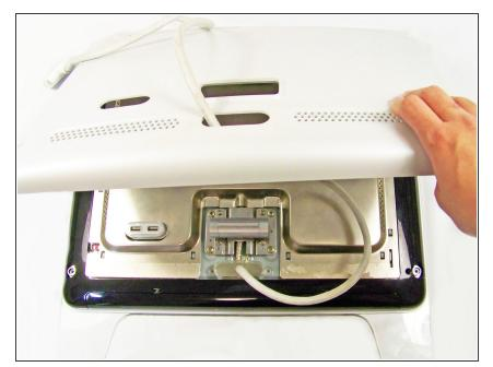
Remove the grey back panel by lifting the bottom and pulling the ADC cable through the hole.
