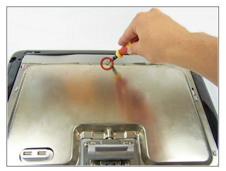
Now locate and remove the lone Phillips screw holding the EMI shield to the display
