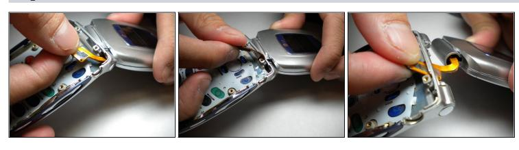
• As shown in the photos, pull the orange strip through a thin opening at the top of the phone. Once this is done, the top and bottom halves can be separated.
