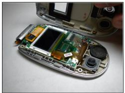
• Carefully open the casing using the iFixit plastic tool by prying each side a little bit at a time. Rotate and open until all the inside clips pop open and the casing opens up.
