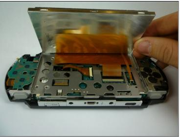
• The LCD Screen is held by the LCD Frame with similar clips. Slide a thin tool between the clip and the screen and gently pry them apart while beginning to lift the screen.
