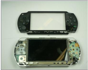
Gently separate the outer plastic casing from the rest of the system as shown.
