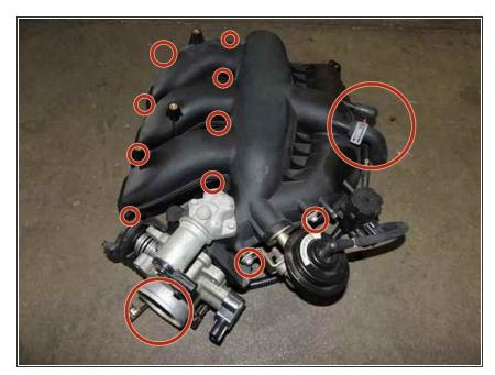
Start removing all the mark parts in red circles. (upper bolts from the intake manifold,hoses,vacuum hoses,filter tube,etc)
