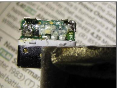
Unsolder the braids and core from both sides of the circuit board.
