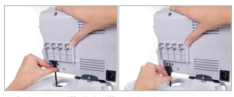
Detach any accessory USB cables from USB ports on the monitor.
