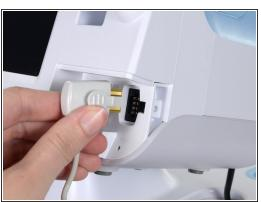
Depress the spring tab on the temperature probe cable connector and withdraw it from the probe port.
