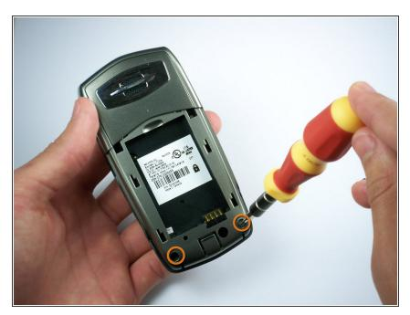
Using the T6 Torx screwdriver, remove the bottom two screws on the back of the phone.
