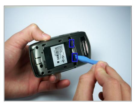
Remove speaker phone cover by unsecuring the two latches on the edge close to top of the phone with the plastic opening tool.
