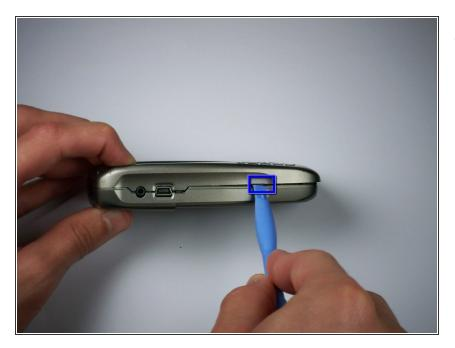
Turn the phone sideways and unlatch the hinge on one side of the phone by pushing inwards and twisting to the side with the plastic opening tool.
