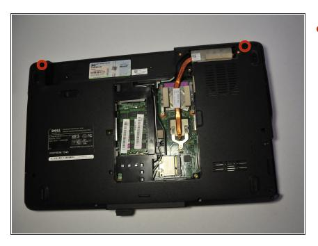
Remove the two screws (5.5mm, Phillips #1) from the laptop base.
