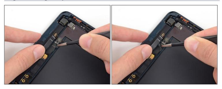
• Use a pair of tweezers to peel up and remove the small piece of tape covering the headphone jack cable connector.
