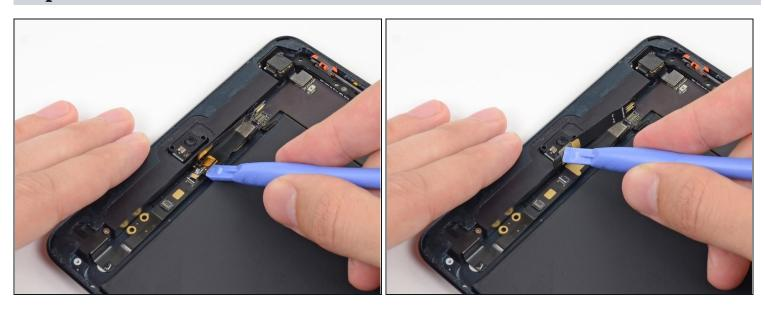
• Gently bend the microphone cable up and out of the way of the headphone jack cable.
