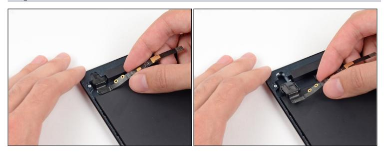
• Pull the headphone jack straight out of its recess in the rear case.
