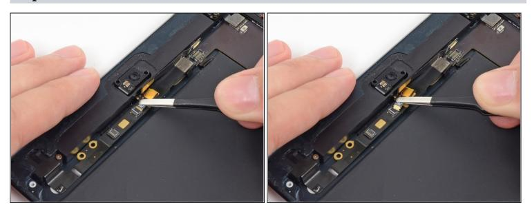
• Use tweezers to pull the microphone cable straight out from its ZIF socket.
