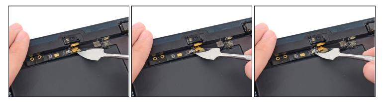
• Slowly work the pointed end of a metal spudger underneath the microphone cable, separating the adhesive securing it to the headphone jack cable.
