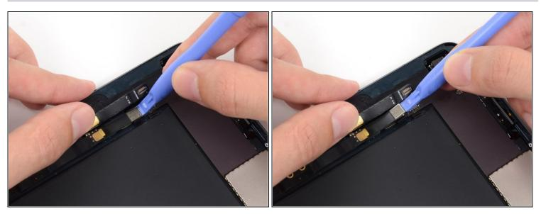
• Use a plastic opening tool to pry the headphone jack cable's connector up from its socket on the logic board.
