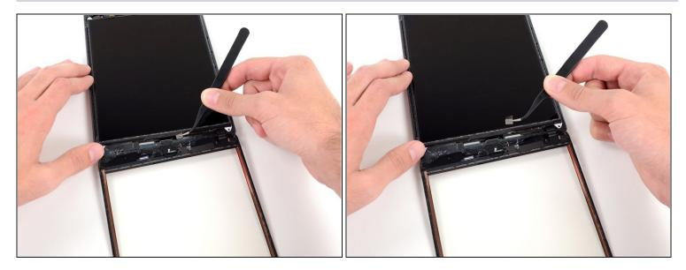
• Use a pair of tweezers to peel up the small piece of tape connecting the LCD frame to the right speaker.
