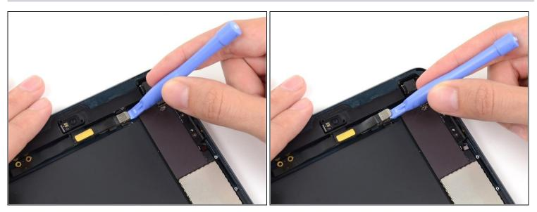
• Use a plastic opening tool to pry the front-facing camera cable's connector up from its socket on the logic board.
