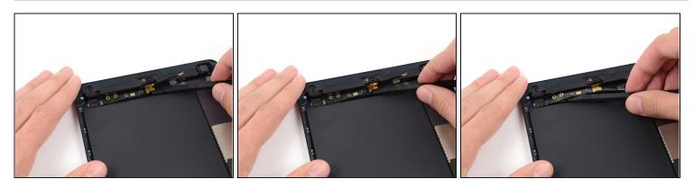
Slide the flat end of a spudger beneath the length of the headphone jack cable, separating the adhesive securing the cable to the rear case.
