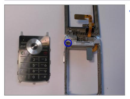
• Remove the small silver screw located where the top of the back of the phone.
