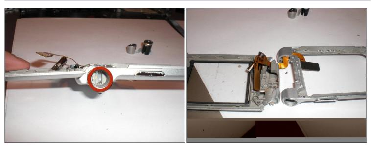
Push in the white thing in the middle, it's spring-loaded, and pull the frame halves apart.
