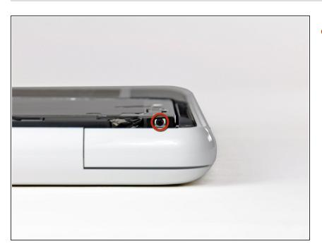
Remove the single 2.2 mm Phillips screw inserted horizontally into the side of the optical drive.
