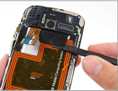
Use the flat end of a spudger to peel the adhesive pull-tab off the top of battery.
