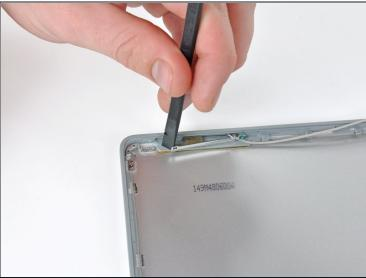
• The antenna is attached to the rear display bezel via adhesive. To remove it, place the flat end of a spudger behind the top edge of the antenna, and carefully twist the spudger to pop the antenna off.
