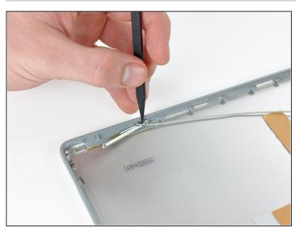
Place the pointed end of the spudger behind the lower part of the antenna and carefully rotate the spudger to free the antenna from the rear display bezel.
