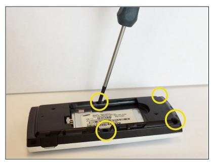
Use a Phillips #00 screwdriver to unscrew the four 3/16" screws holding the black plastic cover of the phone in place.
