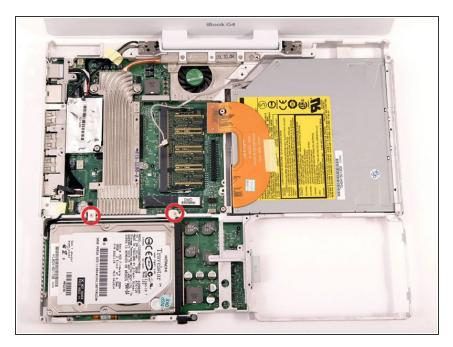
Remove the two Phillips screws securing the hard drive to the metal framework.
