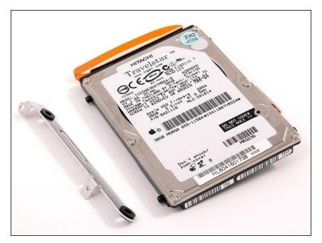
Remove the hard drive bracket from the left side of the hard drive.
