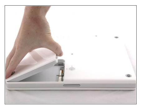
Lift the battery out of the computer.
