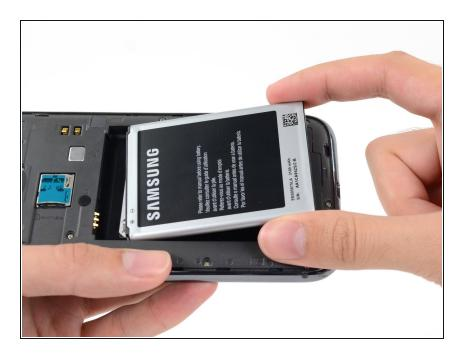
Remove the battery from the midframe.
