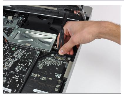
Rotate the display out of the outer case enough to disconnect the LED backlight power cable from the LED driver board.
