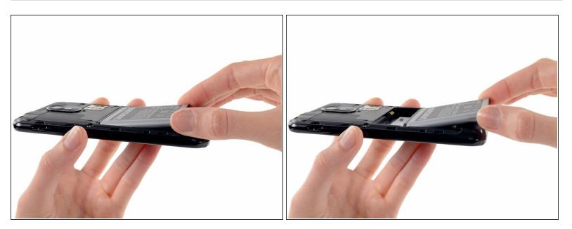
• Lift and remove the battery from the midframe.
