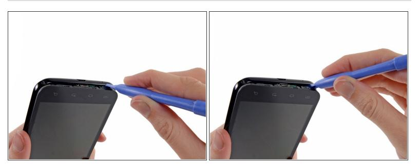
Wedge a plastic opening tool slightly to the right of the micro-USB port, and pry between the midframe and the display to widen the gap.
