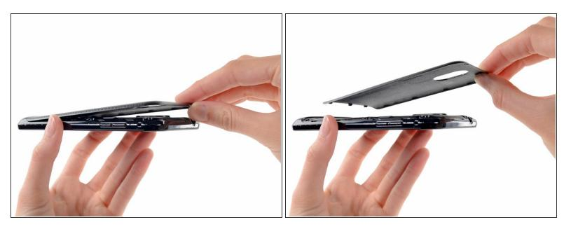
• Lift and remove the rear case.
