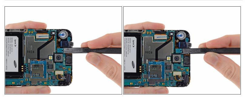
• Use the flat end of a spudger to disconnect the headphone jack/vibrator assembly cable.
