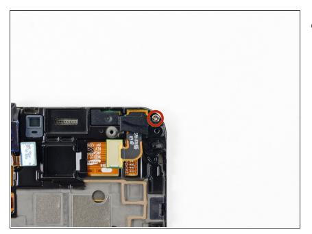
Remove the 2.3 mm Phillips #00 screw securing the front-facing camera bracket to the display assembly.
