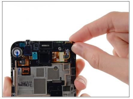
• Remove the front-facing camera bracket from the display assembly.
