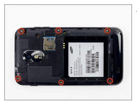
Remove the six 4.0 mm Phillips #00 screws securing the midframe to the front panel assembly.
