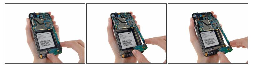
• Lift the micro-USB end of the motherboard away from the display assembly and pull it down.
