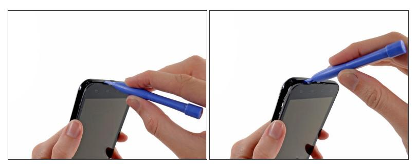
Insert a plastic opening tool slightly to the left of the micro-USB port, and pry between the midframe and the display to open a gap.
