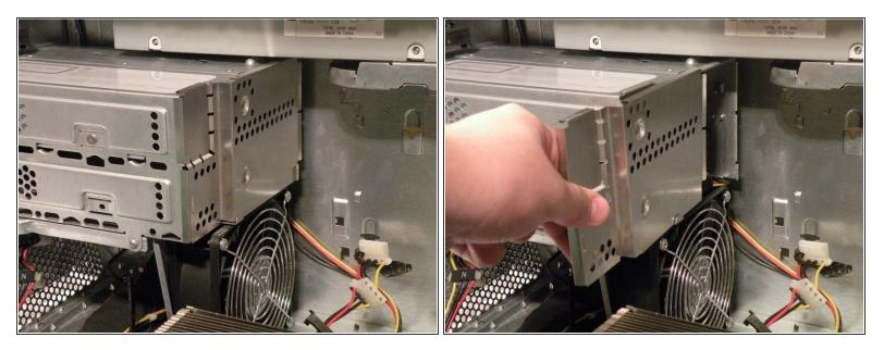
• Start removing the optical drive cage by removing its back cover.
