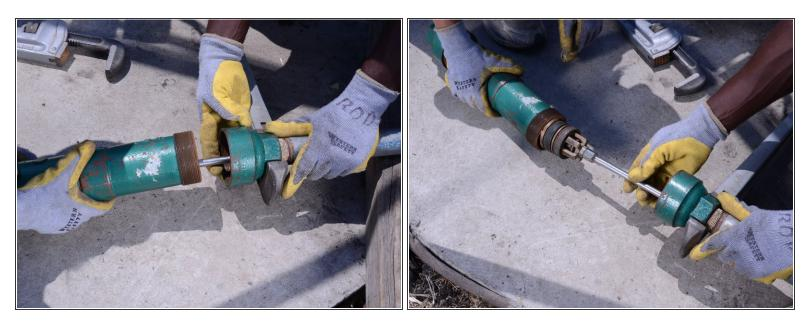
• Slowly pull the cylinder off of the pump rod, exposing the traveling valve and foot valve.
