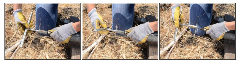
• Remove the T-handle from the top of the pump rod.
