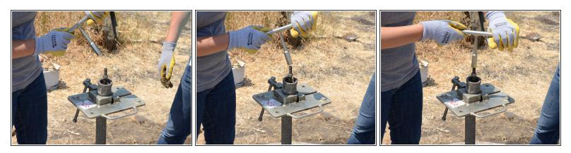
• Reattach the T-handle to the top of the pump rod.
