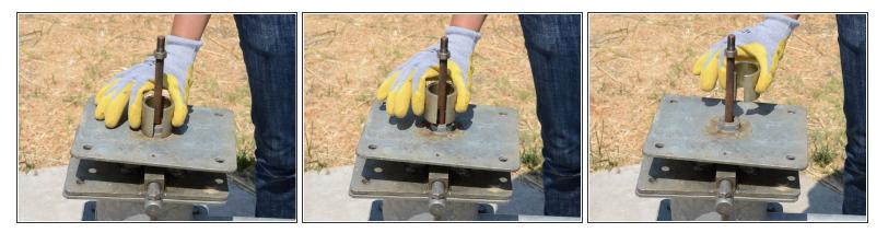
• Remove the chain support from around the pump rod.
