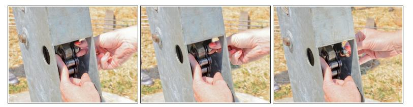
• Remove the nut from the chain bolt.
