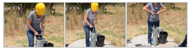
Use the T-handle to pull the pump rod straight up out of the well.
