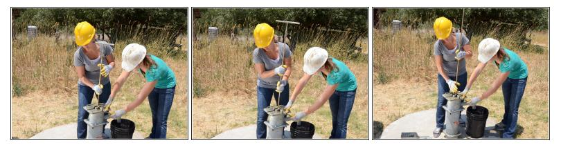
• Loosen the rod clamp and repeat the procedure for the next section of pump rod.
