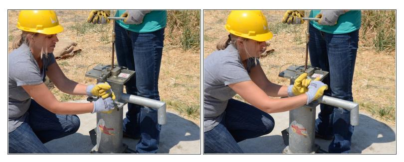
• Have one team member lightly pull up on the T-handle, while another loosens the rod clamp. This will prevent damage to the pump.
