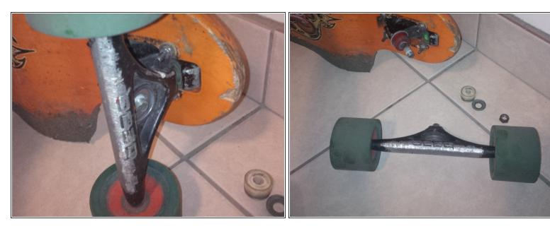
Pull the hanger (horizontal metal bar attached to the wheels) out of the pivot cup and off of the kingpin bolt and set it aside.
