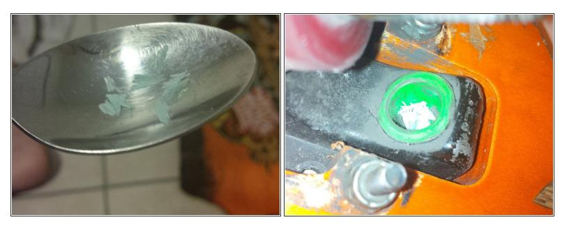
Scrape off a small amount of bar soap and place it in the pivot cup (the green hole in picture 2)
