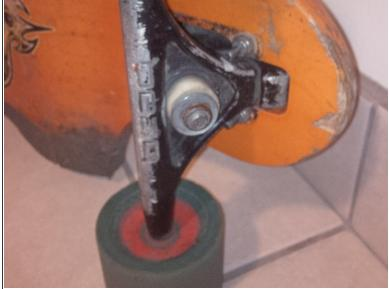
• After you have added on the washer, screw on the kingpin nut and tighten to preference. The tighter the nut the stiffer the turning capability, so this is personal preference. Usually I find that screwing it on until 1 or 2 threads of the kingpin bolt are visible above the nut is sufficient.
