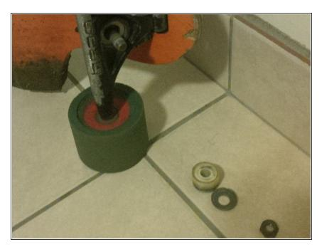
Pull off the white rubber bushing and set it down next to the washer.
