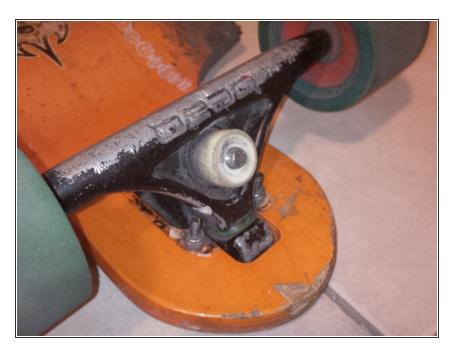
Put the white rubber bushing back on the kingpin bolt, followed by the washer.
