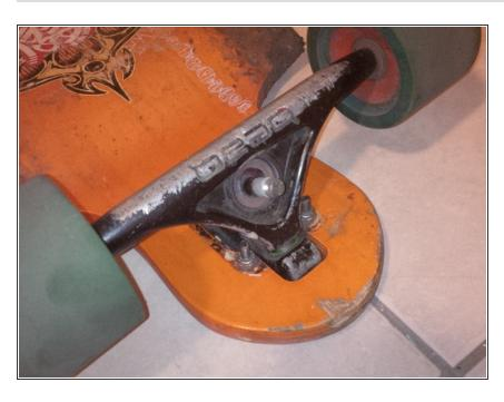
Insert the hanger back onto the kingpin and into the pivot cup and work it around a little bit to spread the soap
