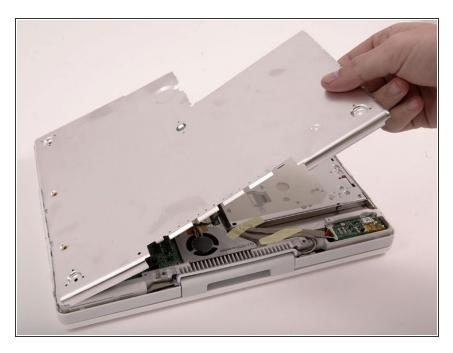
Lift the bottom shield off.
