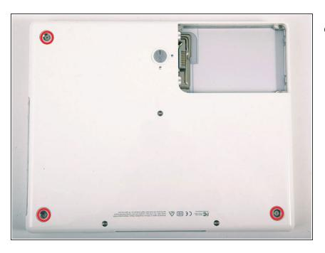
Remove the three newly-revealed Phillips screws.
