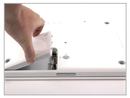
Lift the battery out of the computer.
