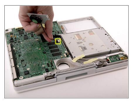
Lift the fan out of its compartment and disconnect it from the logic board, removing tape as necessary.
