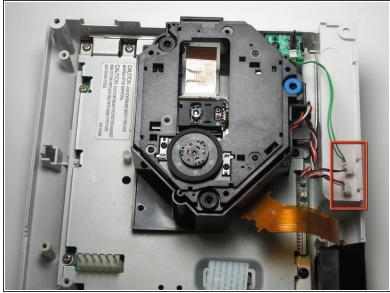
Detach the cables by gently pulling the three GD-ROM cables to remove them from the logic board.
