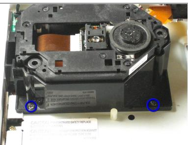
Secure the new GD-ROM drive to the console with the Philips #2 screws.
