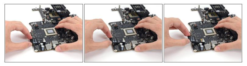
To avoid damaging its socket, do not lift the end of the AirPort/Bluetooth Card excessively.
