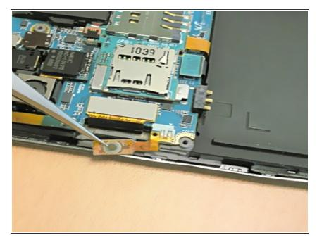
Detach the Power Key FPCB, that is stick to the bracket by a doublesided tape, using tweezers. Make sure to remove all remaining tape on the bracket.
