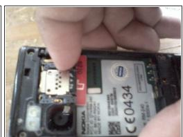
Press the eject button to open battery enclosure. Remove battery, sim card and micro sd card.
