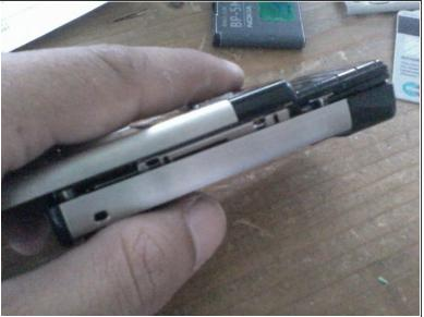
• The top and bottom half of the phone is still connected by two ribbon connectors each side. Use a thin plastic like a credit card to carefully disconnect it.
