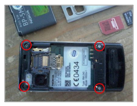
Remove four screws using torx 5 screwdriver.
