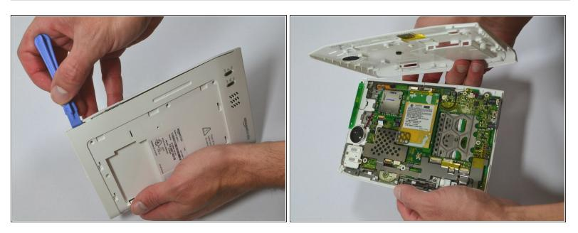
Start at one side of the device. Use a plastic opening tool to separate the casing of the device.
