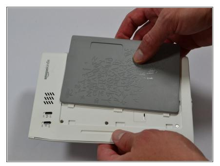
• Slide the grey plastic cover laterally off the back of the device.
