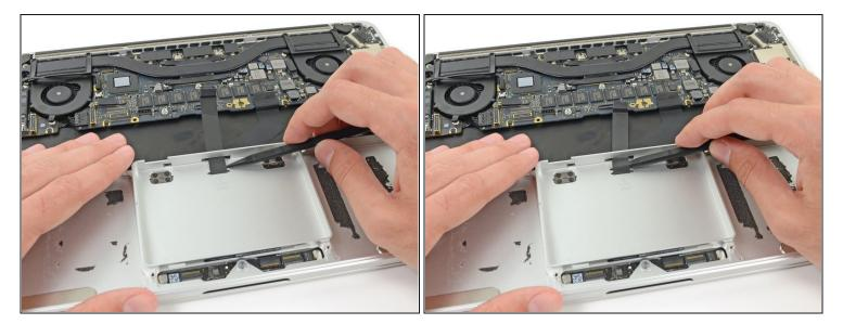
• Insert the tip of a spudger in between the trackpad ribbon cable and the upper case inside the SSD assembly cavity to remove the last of the adhesive.
