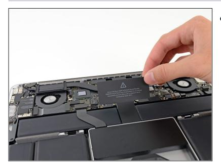
• Remove the plastic cover adhered to the battery contact board.
