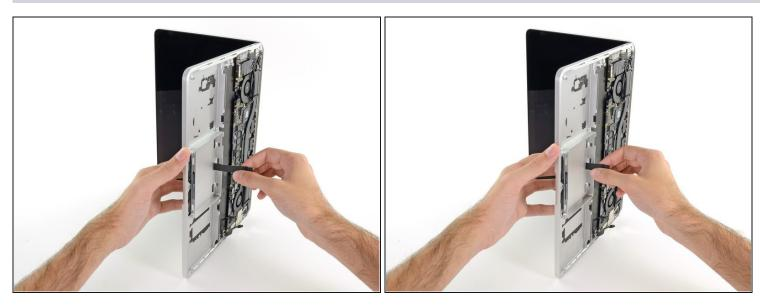
(i) To avoid scratching the display, open the computer about 90° and set it on end.
