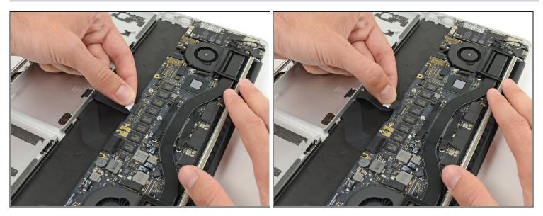
• Grasp the plastic pull tab and pull the trackpad ribbon cable out of its socket.
