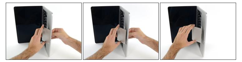
• Gently pull the trackpad from the upper case, being careful not to snag the ribbon cable.
