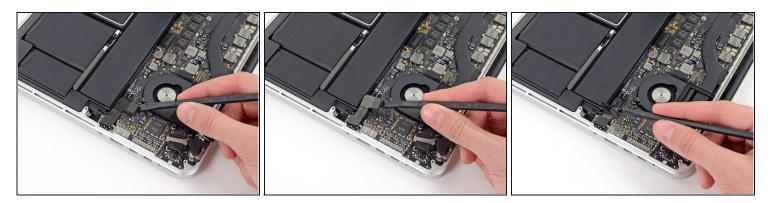
• Use the flat end of a spudger to pry the headphone jack cable connector straight up off its socket on the logic board.
