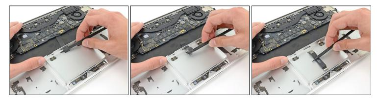
• Using the tip of the spudger carefully thread the trackpad ribbon cable out of the notch near the top of the SSD assembly cavity.
