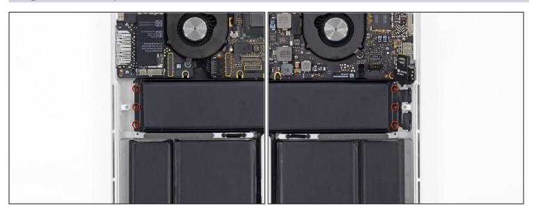
• Remove three 2.2 mm T5 Torx screws from each side of the battery (six screws total).
