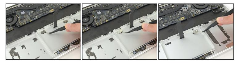
• Use <u>tweezers</u> to remove the two trackpad mounting brackets from the upper case.
