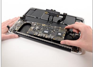
Carefully grasp the corner of the logic board (opposite of the I/O ports) and lift the logic board out of the upper case.
