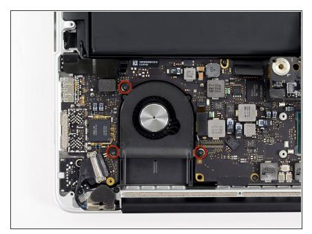
Remove the three 3.1 mm T5 Torx screws securing the left fan to the logic board assembly.
