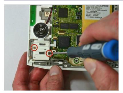
Remove the two (2) Phillips #00 screws (3 mm) connecting the ON/OFF Power and Wifi Switches.
