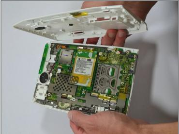
• Start at one side of the device. Use a plastic opening tool to separate the casing of the device. Slowly work your way around the entire device.
