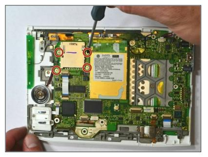
Remove the four (4) Phillips #00 screws (3 mm) which fasten the SD Card Reader.
