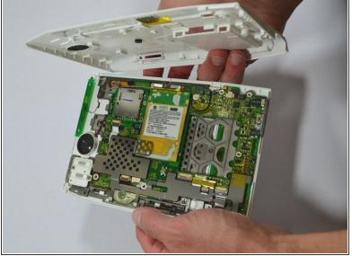
Start at one side of the device. Use a plastic opening tool to separate the casing of the device.
