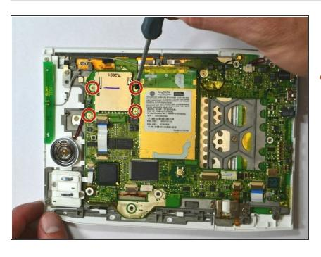
Remove the four (4) Phillips #00 screws (3 mm) which fasten the SD Card Reader.
