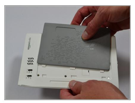
Slide the grey plastic cover laterally off the back of the device.
