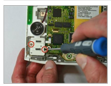
Remove the two (2) Phillips #00 screws (3 mm) connecting the ON/OFF Power and Wifi Switches.
